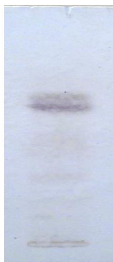
Figure 2: HPTLC Chromatogram in day light after derivatization
